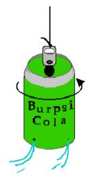
TOPIC: Newton's Laws of Motion OBJECTIVE: Rocketry DESCRIPTION: Water streaming through holes in the bottom of a suspended soda pop can causes the can to rotate. CONTRIBUTED BY: Tom Clausen, KSC Explorations Station EDITED BY: Roger Storm, NASA Glenn Research Center
