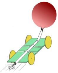
TOPIC: Newton's Third Law of Motion OBJECTIVE: To construct a car to demonstrate how rockets move by means of action and reaction. DESCRIPTION: A small car is propelled by the action/reaction force generated by a balloon. CONTRIBUTED BY: Gregory Vogt, OSU EDITED BY: Roger Storm, NASA Glenn Research Center
